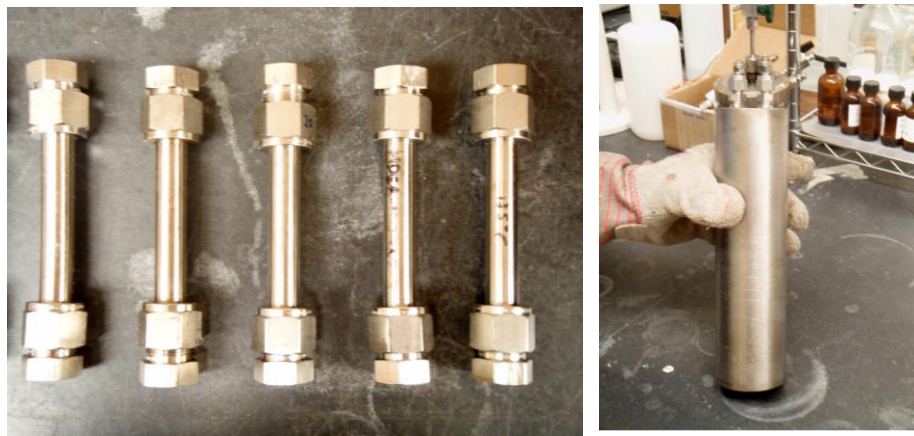
Figure 3.11: Photograph of stainless-steel pressure vessels
